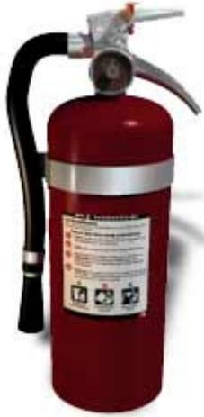
Dry chemical extinguishers put out fires by coating the fuel with a thin layer of fire retardant powder, separating the fuel from the oxygen. The powder also works to interrupt the chemical reaction, which makes these extinguishers extremely effective.
