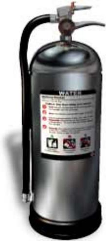
Water is one of the most commonly used extinguishing agents for type A fires. You can recognize an APW by its large silver container. They are filled about two-thirds of the way with ordinary water, then pressurized with air. In some cases, detergents are added to the water to produce a foam. They stand about two to three feet tall and weigh approximately 25 pounds when full.
