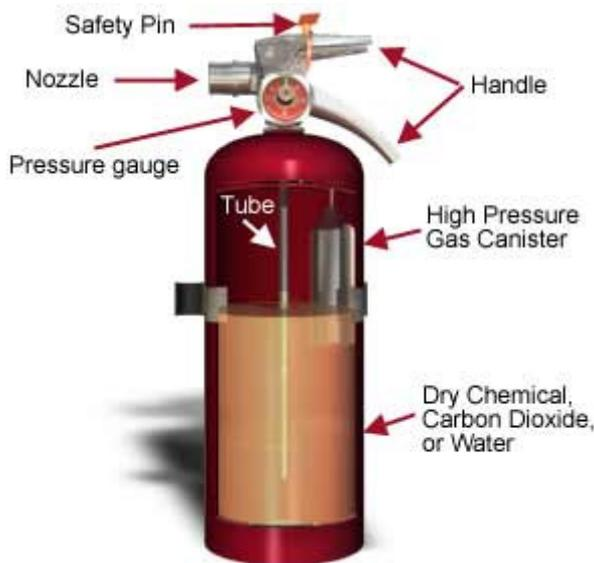
All portable fire extinguishers must be approved by a nationally recognized testing laboratory to verify compliance with applicable standards [29 CFR 1910.157(c)(2)]. Equipment that passes the laboratory's tests are labeled and given an alpha-numeric classification based on the type and size of fire it will extinguish.
